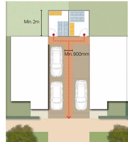
**Figure 26:** Indicative layout of a bicycle and bin storage area at the back of semi-detached properties.
